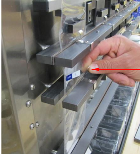
Hook on front part of Clamp Bar C
