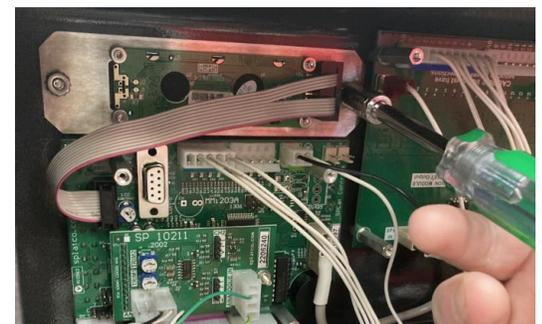
4. Detach the LCD Screen Assembly from the chip board by unclipping the lefthand portion of the connecting wire. Remove the assembly from its position by pulling away gently.
