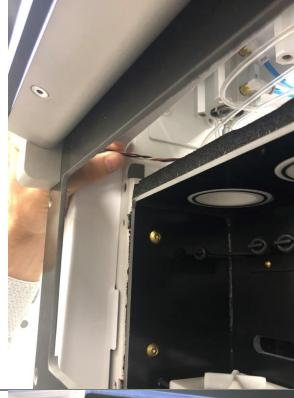
20. Hold the oven face plate in place while screwing in the five screws previously removed.
