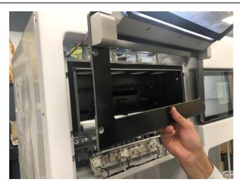
There are wires for the LED lights still connected to the instrument in the upper left corner of the oven face plate.
