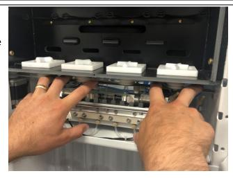
15. Reattach the fluid lines, making sure that they are screwed straight in. BE CAREFUL not to cross threaded.
