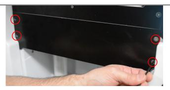
2. Open the digestion oven door and use the 5/64" Allen Hex wrench to remove the center screw on the oven face plate.
