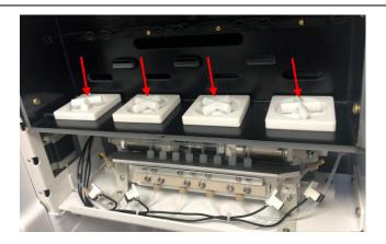
Locate the four retaining clips below the stabilizer plate. Using the 90-degree angled pick, pull the retaining clips off the magnetic spinner shafts and set aside.
