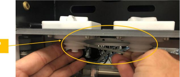
11. Install the new round belts in the colored specified order. Make sure that the belts are completely in the grooves
