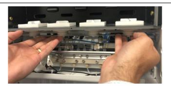
13. Replace the retaining clips into their grooves by pushing them until they are completely against the magnetic spinner shafts.
