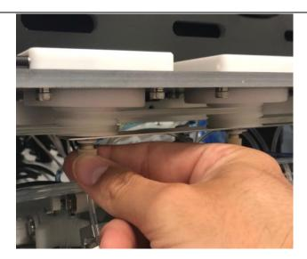
16. Hand tighten the lower tube fittings to ensure that they have not become loose.
