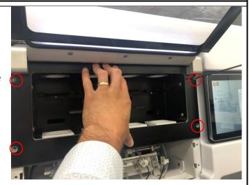
4. Carefully pull the oven face plate away from the instrument but do not completely detach.
