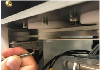
8. Observe the right side of the stabilizer plate and ensure that there is **NO** set screw connecting it to the wall. There <u>should not</u> be a screw, remove if there is one.
