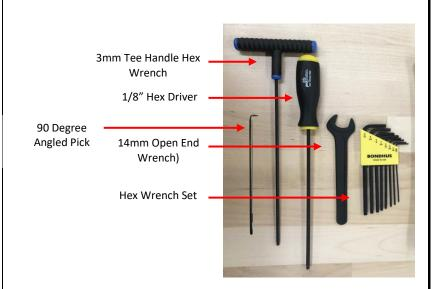
1. Use the 1/8" Hex Driver to remove the four screws on the front access panel, then remove the panel.
