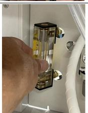
10. Install the new nitrogen flow meter.
