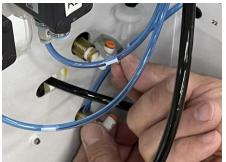
9. Open the reservoir doors and remove the old nitrogen flow meter from the rear of the cabinet.
