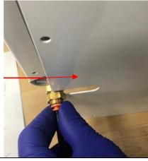
14. Using the 1/8" Hex Driver, reinstall the (20) rear panel screws on the back of the instrument.
