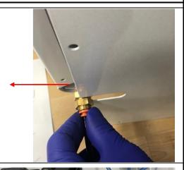
7. In the back left panel of the instrument, remove the two nitrogen wires connected to the flow meter.
