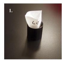
This method uses Celite (diatomaceous earth) in place of weigh tins when testing high fat samples.
