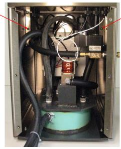
1. Remove the cabinet back and remove the six screws.
