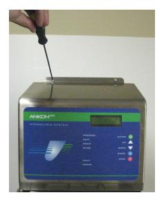
4. Remove the two electrical cabinet screws open cabinet by pulling forward.
