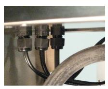
7. Loose each Cabinet Bulkhead Fitting for the wires that are being replaced. Pull the wires through the fittings.
