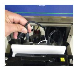
8. Carefully twist and pull and remove the bad Heater Cartridges from the vessel.
