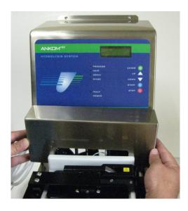
3. Remove the heater cover from the front of the instrument.
