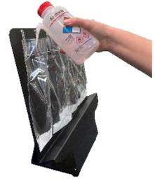
26.4 After the two full rinses, target any sample still clinging to the walls of the bag with Acetone making sure all of the sample is pushed into the filter part of the bag.
