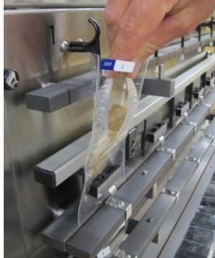
**IMPORTANT:** When adding sample to the IDF *Flow-thru* bags it is very important to keep it below the tip of the Delivery Nozzle so that it can be properly rinsed.
