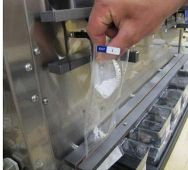
**IMPORTANT:** When adding DE to the filter bags it is very important to keep it below the tip of the Delivery Nozzle so that the DE material can be properly rinsed.
