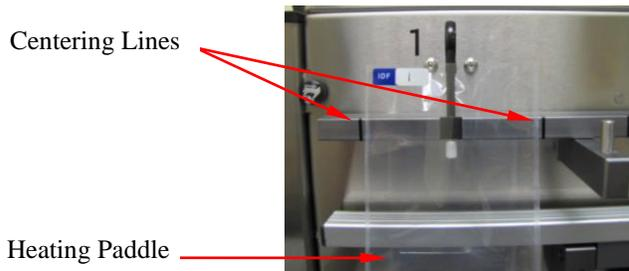
**IMPORTANT:** For proper mixing during the IDF process the IDF bags must be horizontally centered over the Heating Paddles and between the Centering Lines on the back part of Clamp Bar A.
