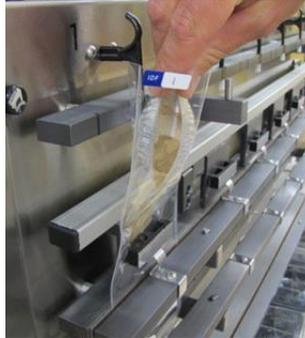
**IMPORTANT:** When adding sample to the filter bags it is very important to keep it below the tip of the Delivery Nozzle so that it can be properly rinsed.
