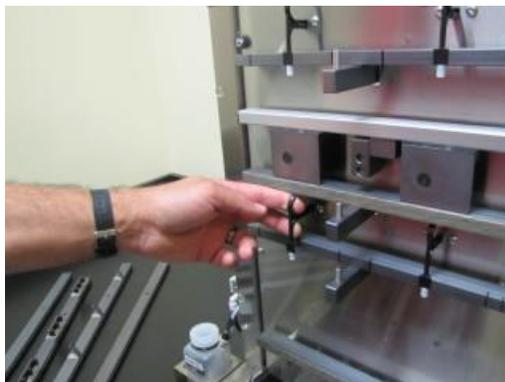
11.3 Place a labeled and weighed SDF bag up underneath the SDF Delivery Nozzle so that the Delivery Nozzle is inside the top part of the bag. Pull the bag up so that the top of the bag is about 35 mm (1.375 inches) above the top of Clamp Bar C and return the Delivery Nozzle to its original position. This will hold the back of the bag in place.
