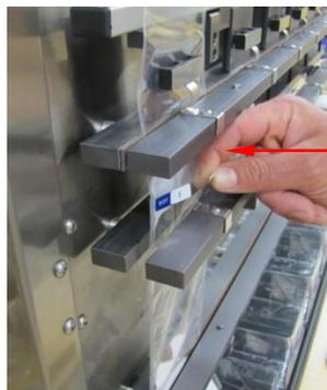
Hook on front part of Clamp Bar C
