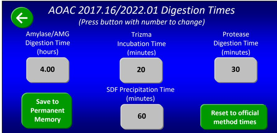
This diagnostic allows you to modify the times used by the computer for the digestion processes. This can be helpful when troubleshooting or demonstrating the instrument. If you press the “Save to Permanent Memory” button, the values you entered will be saved until you change them again by using this diagnostic. If you do not press the “Save to Permanent Memory” button, the values you entered will be saved until power is turned off, or until you change them again by using this diagnostic.
