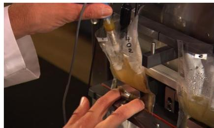
When you have completed the pH measurement process straighten each bag by lifting them back into place. Press the “Continue” button on the Status screen. You will see “COMPLETE” next to “pH Trizma?” in the upper left corner of the screen.
