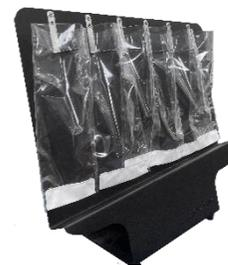
26.3 Using a wash bottle, squirt acetone completely around the inside polypropylene surfaces of each bag two times, making sure that all residue is rinsed down into the filter.
