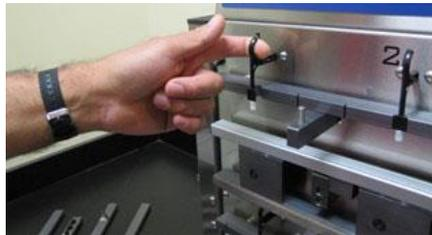
13.2 Place a labeled IDF *Flow-Thru* bag up underneath the Delivery Nozzle so that the Delivery Nozzle is inside the top part of the bag. Pull the bag up so that the top of the bag is about 35 mm (1.375 inches) above the top of Clamp Bar A and return the Delivery Nozzle to its original position. This will hold the back of the bag in place.
