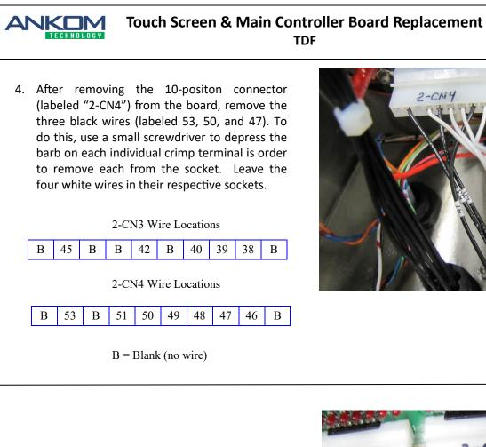
5. Do the same for the 10-position connector (labeled "2-CN3"). The wires to be removed on tis connector are labeled 45, 42, and 39. Leave the other two black wires in their respective sockets.
