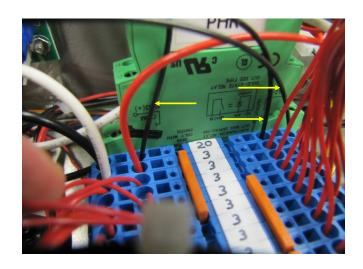
Unplug the two, 10-position connectors (8308) labeled "2-CN4" and "2-CN3" (Yellow Arrows) from the circuit board labeled "I/O2". You may need to use a needle nose pliers to grasp one side and then the other to work these out of there position on the circuit board.
