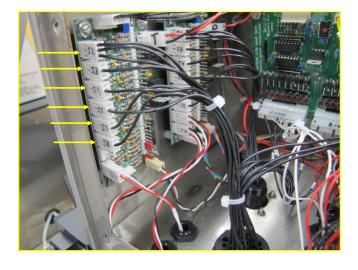
2. Disconnect the three black wires (Yellow Arrows) that are connected into sockets in the #20 terminal blocks on the 24v DIN rail. To remove the wires from the DIN rail it is necessary to insert a small screw driver into the square hole next to the hole where the wire resides and press down to release the latch on the wire. (To insert the replacement wire you will again need to press down with a screw-driver.)
