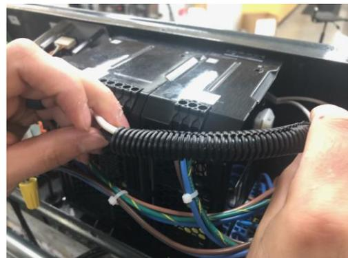
11. Place a zip tie through the white zip tie fastener on the side of power supply A and loosely tighten around the wires being held by the black wire sleeve. Cut off zip tie excess.
