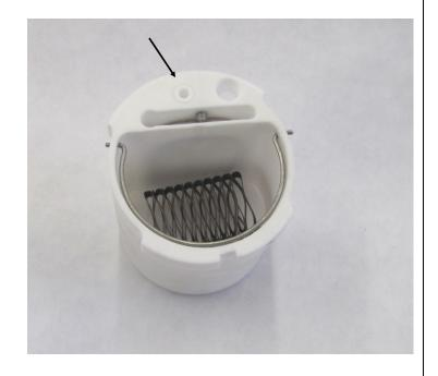
2. The large O-Ring is installed in the Vessel as shown.
