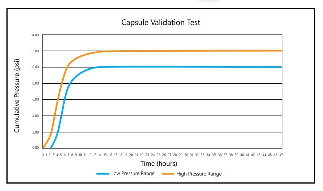
The ANKOM RF Positive Control Capsule Set was developed to simplify the validation test of your RF Gas Production System and provide a positive control curve for comparison between experiments.
