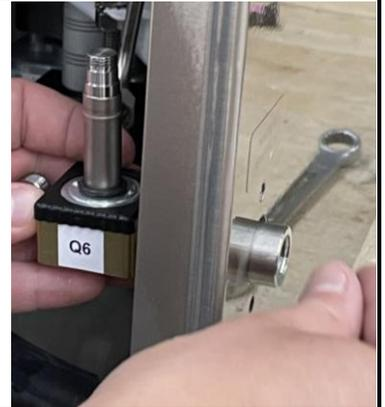
2.6. Replace the pipe onto the water valve and secure in place with the 9/16" or adjustable wrench.
