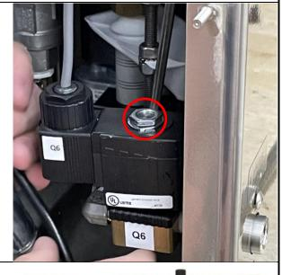
2.9. Reattach the panel and reinstall the nuts that secure the back panel of the A2000 with a 3/8" wrench. Plug the instrument back in and power on.
