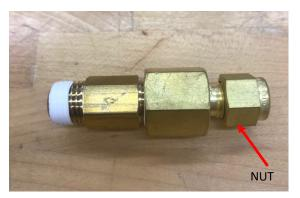
2. If an A13 Copper Tube Assembly was purchased, the nut (Red Arrow) comes already installed on the Copper tubing. Remove the nut from the A07 Water Filter (This is an extra and can be saved in case the one being used is damaged) and use the one already installed on the Copper tubing Assembly. When connecting it to the A07 Water Filter, Take notice of the direction of the ferrule (Blue Arrow).
