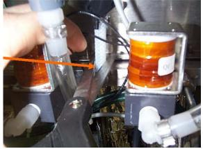
2. Turn the old fitting counterclockwise to remove. Screw the new stainless fitting on by hand and then 1-2 more turns with the wrench to make the fitting vertical. Note: If you are unable to turn the fitting all the way to vertical, unscrew it, remove the Teflon tape and re-tape it with an extra layer of Teflon tape so that you do not have to turn it in as far to get a good seal.
