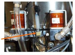
1. Cut the pressure switch tube just above the bottom clamp. You will re-use the rest of the tube. Be careful not to cut any wires!
