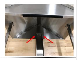
6. Remove six nuts from the back of the A2000 (red arrows).
