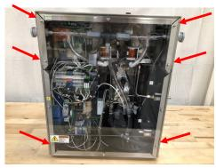
7. Slide on the Left and Right Support Brackets and the Triangular Back Brace as shown (red arrows), then replace the nuts. Adjust the Leveling Foot (blue arrow) as needed to support the bracket. The foam strip should rest on the top of the A2000.
