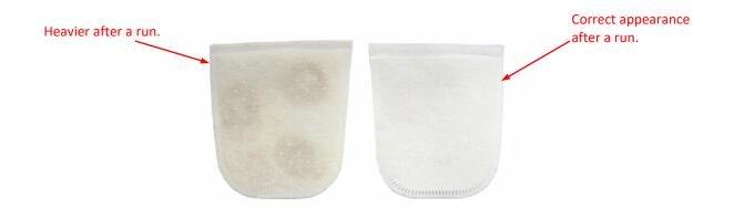
Generally, the best way to determine if sample has been lost is to examine the blank bag weights. If the blank bag is heavier after the run than it was before, fine particles have escaped from the filter bags during the extraction process. To correct this problem, use the recommended grinding options referred to above.
