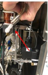
5. Disconnect the clear tubing from the barbed fittings on the quick-disconnects at the outside wall of the instrument.
