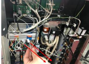
**5.** Remove the six-position connector from the pressure sensor and tube end. Then, begin to install the new DELTA17 by first replacing the tube and pressure sensor end.
