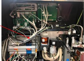
3. Cut the zip ties holding the DELTA17's in place and isolate the one that needs replacing.
