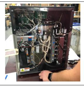
2. Locate the two DELTA17 pressure sensor assemblies.
