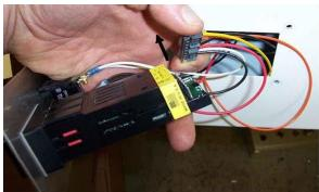
4. Remove the controller from the plate by spreading the retaining clips apart (spread the clips on both sides) and pulling the controller out of the front of the plate.
