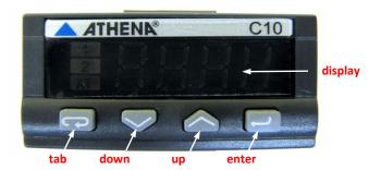
The Athena Controller (shown above) maintains the proper temperatures within the D200/D200I. To configure the controller, follow the procedure below. If you make a mistake at any point in the procedure, go back to step 2 and start over.
