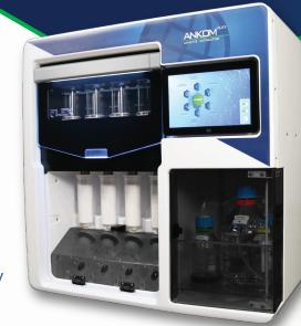
The ANKOM<sup>FLEX</sup> Analyte Extractor is designed to simplify fat-soluble vitamin, cholesterol, and crude and hydrolysis fat determinations. Supporting up to four samples at a time, the system will automatically complete digestion, solid phase extraction (SPE) and evaporation in about two to three hours.
