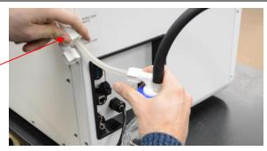
3. Connect one of the 10 ft opaque exhaust tubes to the waste assembly exhaust line connection. Make sure the tube is pushed all the way into the exhaust line before hand tightening the nut onto the tube.
