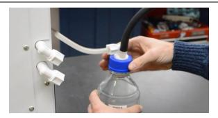
Connect the shorter opaque tube to the Vessel Vent on the left side of the instrument. Make sure the tube is pushed all the way into the port, then tighten the white nut finger tight.
