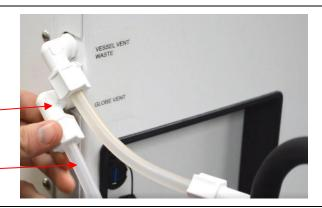
5. Vent both exhaust tubes to exhaust system.
