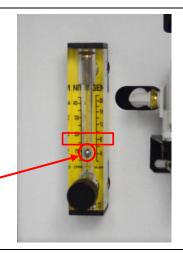
5. When the float has been adjusted to be within the acceptable range, turn the Globe N2 "Off."
