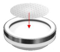
2. Wet the bottom outside edge of the digestion vessel with water.
