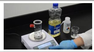
2. Add 9.5g water into the digestion vessel.
