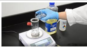
3. With a pipette, add 0.5g oil sample into the digestion vessel.
