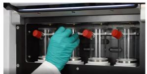
4. Repeat for each vessel you wish to insert the internal standard.
