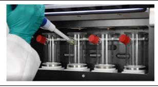
3. Screw the red cap onto the vessel port. Tighten but do not over tighten.
