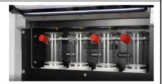
2. Using a pipette, add the internal standard into the digestion vessel through the vessel port.
