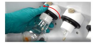
2. Remove the round bottom flasks and immediately cover each flask with aluminum foil or a stopper to protect the analyte.
