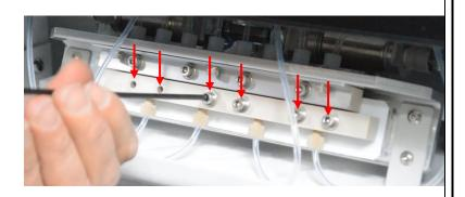
7. While wearing gloves, pull the lower bar forward and inspect the top surface for residue.
