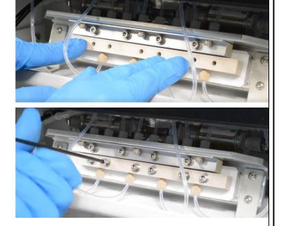
Loosen the three vertical screws until the gap reappears between the metal plates. The washer on the screw should be able to move freely once loosened.
