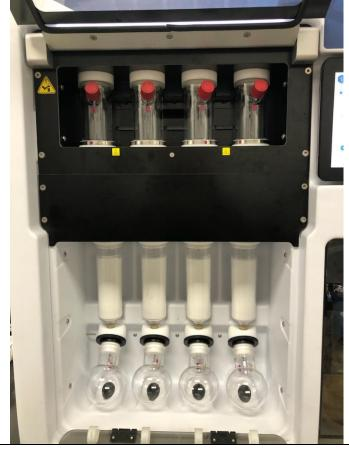
2. Navigate to the command center on the HMI. Close Vessel Tops and Close Column Lock.
