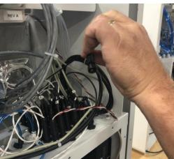
15. Before screwing in the new connector, re-apply any zip ties that were removed.
