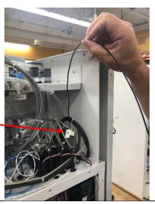
13. Install new liquid sensor. Gently clip the sensor onto the tube in the front of the instrument. Make sure the tubing properly enters the black plastic clip.
