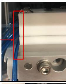
18. Verify that the two nuts on the air cylinder are both tight against the bracket.
