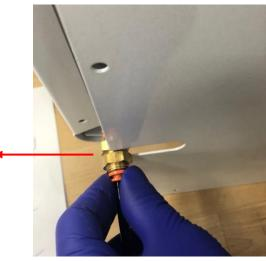
7. Locate the vent valve near the top of the instrument.
