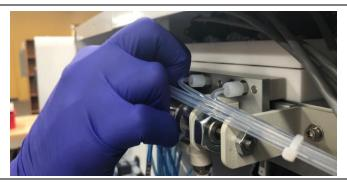
20. Loosen the four screws on the connector plate until the gap reappears between the plate and the slide bar. The washer on the screw should be able to move freely once loosened.
