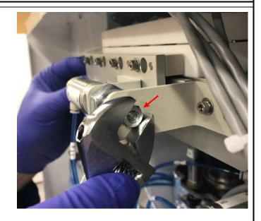
11. Slide the connector plate to the left to remove it from the Instrument.
