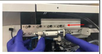
12. Inspect the slide bar for residue. If residue is present, clean the bar using a paper towel dampened with distilled water. Wipe until clean. Do not use any sharp objects which may damage the seals.
