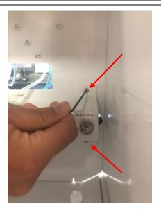
Detach the ¼" (black) nitrogen supply tube, push the orange connecter ring located on the regulator side of tube and move the regulator to the right.
