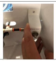
7. Mount bracket onto back wall in reservoir area by reinstalling and tightening the (2) mounting screws.
