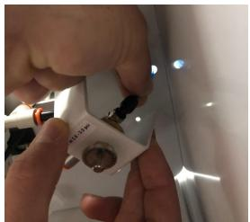
If there is a loop in the nitrogen line, make sure you retain the loop when reconnecting the regulator. If N2 tube is straight then you do not need to add this loop in the nitrogen line.
