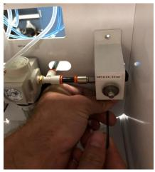
May need to flex bracket to align (2) screw holes.
