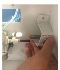
Detach the 4mm (blue/yellow) nitrogen tube, push the black connecter ring located on the regulator side of tube and pull the tubing out of the fitting.
