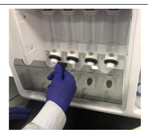
While wearing gloves, unscrew all four of the nozzles. Hold onto the Teflon tube so that it does not spin.
