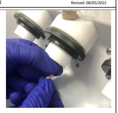
The Teflon tube may have been pulled out. Make sure the Teflon tube is pushed all the way back into the Teflon holder.
