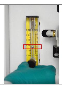
From the command center screen on the HMI, turn globe nitrogen on. Observe the globe pressure.
