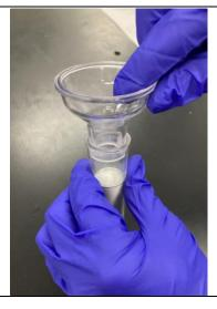
Before installing each SPE column onto the instrument, wipe the inside of the column top (vitamin) or column funnel (fat) and the column top adapter O-ring.
