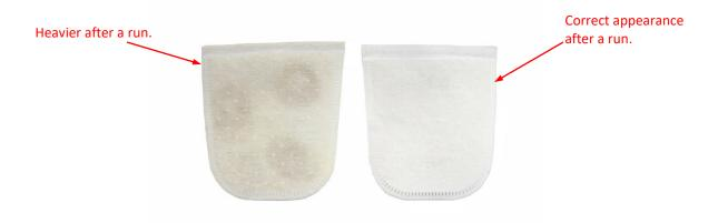
Generally, the best way to determine if sample has been lost is to examine the blank bag weights. If the blank bag is heavier after the run than it was before, fine particles have escaped from the filter bags during the extraction process. To correct this problem, use the recommended grinding options referred to above.
