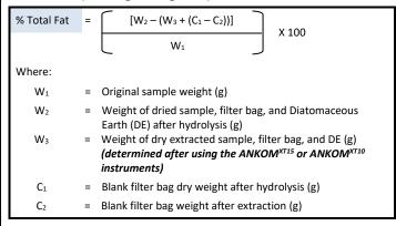
**HCl Procedure** (see the Hydrolysis Procedure section of the Operator's Manual for more detail)
