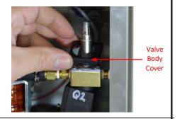
14. Reinstall the Solenoid over the valve guide tube.
