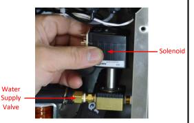
5. Remove the valve body cover from the valve guide tube and set the cover aside.
