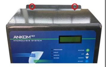
3. Remove the control panel plate cover by removing the four screws with a small Phillips screwdriver.
