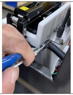
6.2. Reach in through the rear of the instrument and pull the hose off the nozzle it is attached to.
