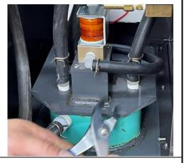
19. On the front left side of the electrical cabinet, install the new hose and hose clamp.
