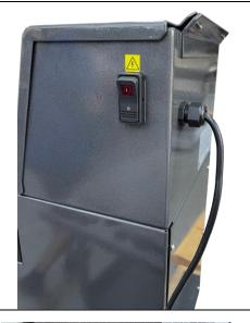
2. Remove the six screws on the rear plate of the instrument using a Hex 1/8" driver.
