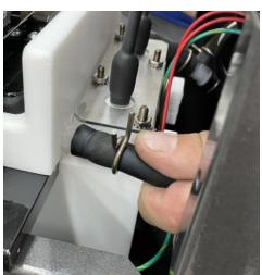
6.3. Pull this portion of the hose through the back of the instrument and let hang to the side as shown.
