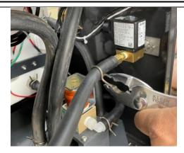
21. Install the hose on the back of the electrical plate, at the front right side of the instrument.
