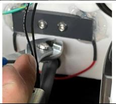
16. Using the same process as step 18, install the new 13" hose on the nozzle located at the far back of the electrical cabinet, toward the front of the instrument.
