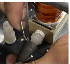
13. With all hoses unplugged from the instrument and set aside, acquire a new #H38 HCl Hose Kit for reassembly.
