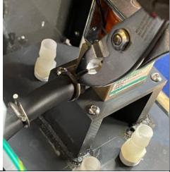
15. Install the other end of the 4" hose located against the back wall of the electrical cabinet.
