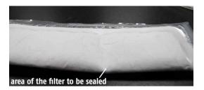
**3.** To seal the filter, the heat sealer should be set to 5. With the filter in place on the heat sealer, the arm of the sealer is pressed down. A click will be heard and the red light will be lit. It is at this time the heat is on. In a second or two, another click will be heard and the light will go off. At this point the heat is deactivated but the sealer arm should remain pressed down for 3-4 more seconds to allow the filter material to cool.
