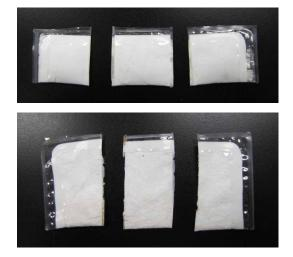
**6.** The three portions of the bag are now each placed in their own crucible in the Teflon sample tray and heated to 120 °C for 30 minutes. While still hot, the bags are pressed into their crucibles with the steel pressing tool to remove any air that would contribute to the blank.
