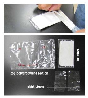
**2.** The next step is to heat seal the two layers of the filter together to create at least three equal sections of filter. The SDF filter contains not only sample residue but also DE. The filter needs to be manipulated so that the mixture is away from the area to be sealed.
