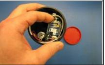
4.1. Lift gently on the bottom left corner of the chip until the corner lifts slightly from the circuit board.
