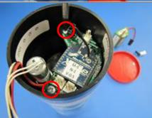
3.4. Remove the old circuit board and chip and install the replacement components.
