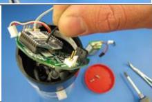
3.5. Repeat steps 3.4 through 3 in reverse order, screwing the circuit board back in place, reconnecting the two-wire solenoid connector, the three-wire pressure sensor connector, and the temperature sensor.
