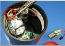
3.2. For RF1/RF1X Modules disconnect the two-wire solenoid connector from the circuit board.
