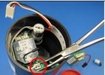
3.3. With all the connectors removed from the circuit board remove the two screws holding the circuit board in the housing, as shown in image right.
