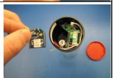
The #RF45X does not have an antenna. In this case, the sides of the #RF45X can be wiggled back and forth until the #RF45X pops out.
