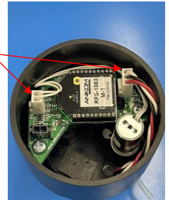
Pressure Sensor and Solenoid Wires
