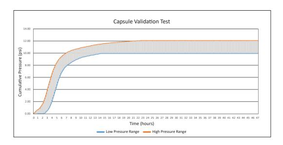
The ANKOM RF Positive Control Capsule Set was developed to simplify the validation test of your RF Gas Production System and provide a positive control curve for comparision between experiments.
