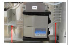
3. Open the Pump doors by pulling on the two latches on the right side of the pump, allowing access to the pump tubing.
