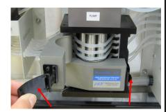
4. Remove the six pump tubes by pulling back on the white stops on the right and left sides of the tubing comb.
