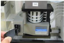
7. Connect the tube end to the barbed fittings on the left and right sides of the pump as shown by the arrows.
