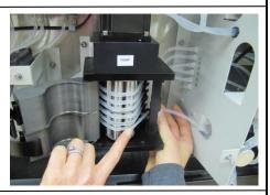
6. Close the Pump doors and snap the latches in place.
