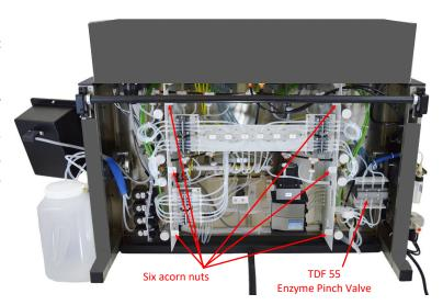
NOTE: It is recommended that when ordering a new TDF55 Enzyme Pinch Valve, that a new TDF67 Enzyme Tubing Set is also ordered.
