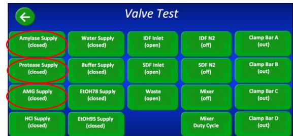
e. Technician #1 presses the “Amylase Supply” button on the Display until the button shows “(closed)”.
