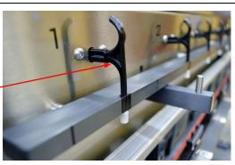
5. Reinstall the spring onto the metal tube and over the molded black plastic by pushing it back all the way.
