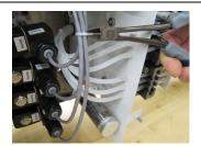
3. Remove the nut from the valve coil that needs replacement. (In this demonstration, the Water Supply Valve Seat and Valve Body Seal will be replaced.)
