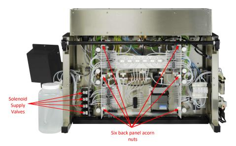
To replace the Valve Seats and Valve Body Seals in the solenoid supply valves on the ANKOM TDF Dietary Fiber Analyzer, follow the steps below.
