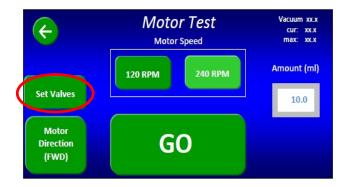
22. Select the Supply valve or valves that have been replaced to be the OPEN valve being tested. (RED ovals) Close all other Supply Valves. This has to be done one at a time. Select the IDF Inlet (GREEN oval) as the open Output valve; close the others. Place beakers or cups under IDF fill nozzles to catch the fluid delivery. Press the left arrow ←
