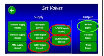
Press GO and confirm that approximately 10 mls of the specified solution has been delivered through the IDF fill nozzles and into the beakers. Confirm that the valve(s) being tested are opening also by observing that the vacuum reading (max) is in the -0.8 to -3.0 psi range. A vacuum greater than -3.0 psi indicates a partial blockage. A vacuum greater than -5.0 psi will present as a plugged line, which could indicate a valve that is not opening.
