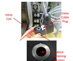
5. Remove the valve body cover from the valve guide tube and set the cover aside.
